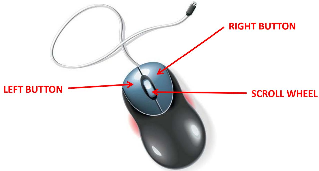
A mouse is a pointer and an input tool that is attached to your computer. It allows navigation around the computer screen. There are different kinds of mice that use different technologies.
