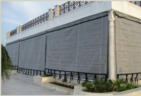
Figure 4-19. Polyethylene basket weave fabric windscreen deployed at edge of patio, enclosing the entire area. Source: Roll-a-way/QMI.
