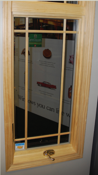
Figure 4-20. This attractive window can be fitted with energy-efficient glass, impact-resistant glass or both. The impact-resistant glass consists of a laminate or film sandwiched between two glass panes. The frames are reinforced, and the hinges have extra fasteners to withstand high wind events. During a wind event, debris may crack the glass, but the laminate will hold the window pane together in the frame and prevent breaching of the wind- and rain-resistant envelope. After the storm, damaged glass will need to be replaced.
